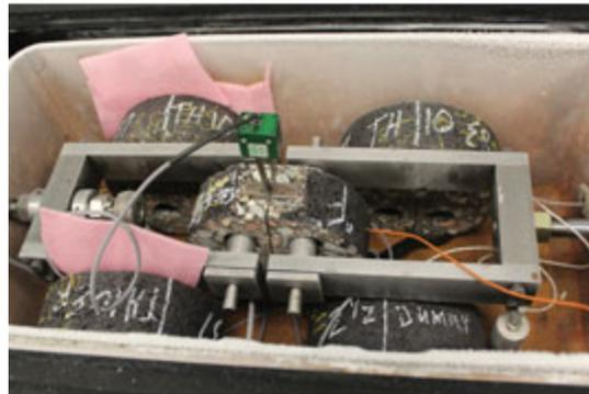
Disk Shaped Compact Tension Testing (DCT) (photo
