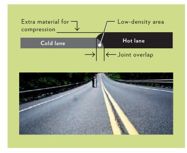
Top: A cross-section of a longitudinal joint reveals the potential for low density and weak spots. Bottom: Poor performance along a longitudinal joint. (Images courtesy of Steve Muench [top], NCAT [bottom])
