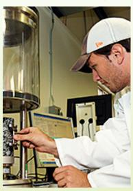
The Asphalt Mixture Performance Tester provides input data for mechanistic-empirical pavement design. (Image courtesy of NCAT)
