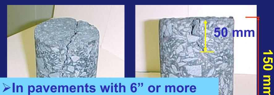
In pavements with 6" or more thickness, longitudinal cracking started at surface
