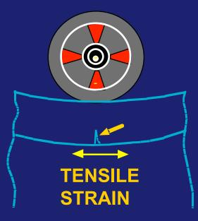
Preventive seals on these pavements mask structural distress and lead to full depth failures
