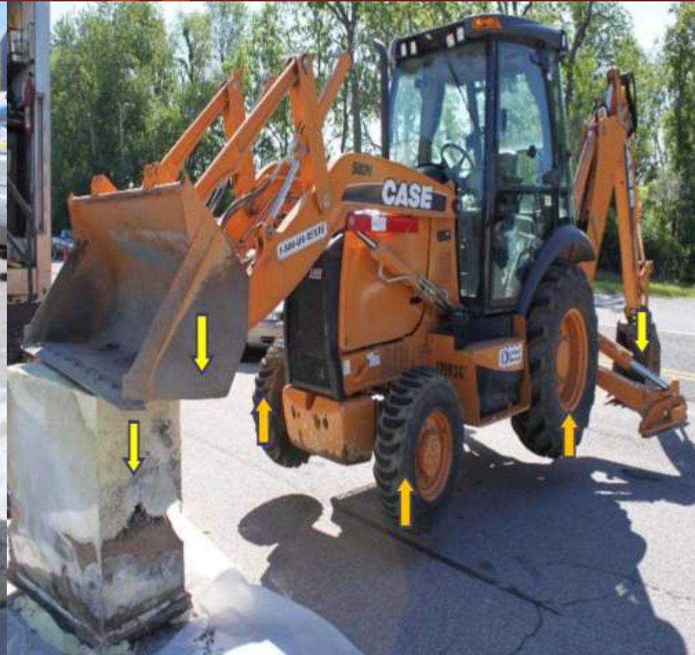
Ad-Hoc Geo-Material/Polymer Matrix Compression Test
