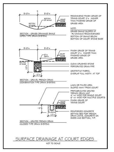
Figure 6. Surface drainage at court edges.<sup>5</sup>
