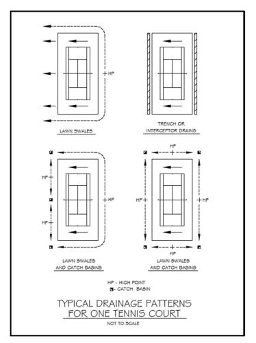
Figure 5. A diagram of tennis court drainage designs.
