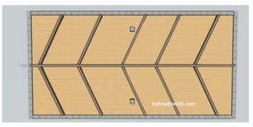
Figure 8. An illustration of drain tiles placed in a herringbone pattern.<sup>7</sup>
