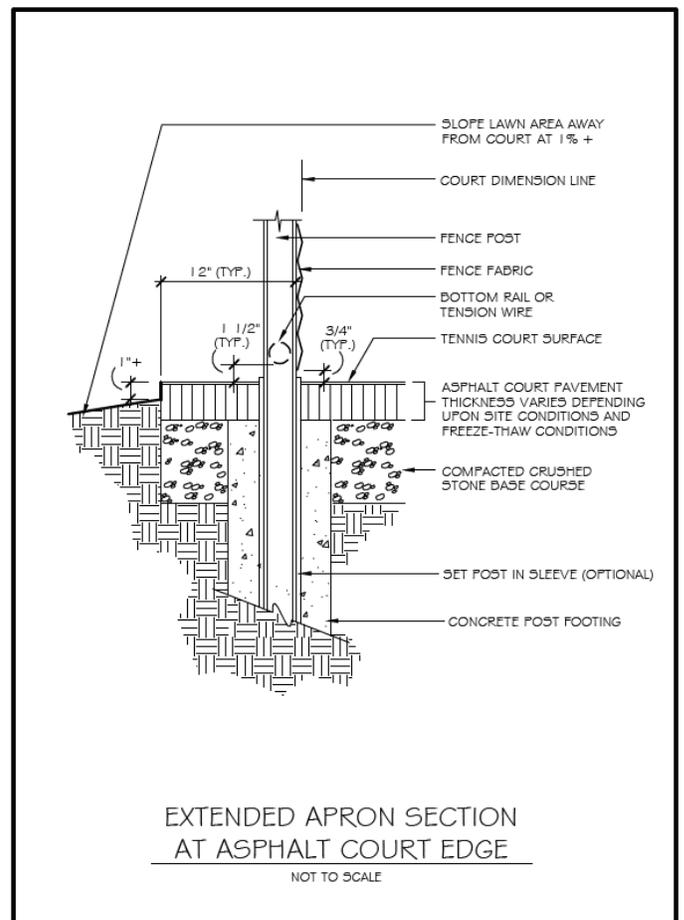
Figure 12. Extended Apron Section at Asphalt Court Edge.
