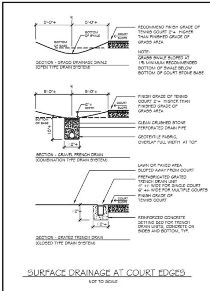
Figure 6. Surface drainage at court edges.<sup>5</sup>
