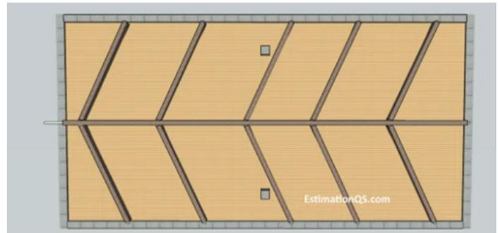
Figure 8. An illustration of drain tiles placed in a herringbone pattern.<sup>7</sup>
