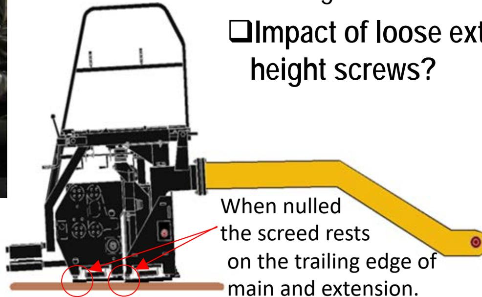
When nulled the screed rests on the trailing edge of main and extension.
