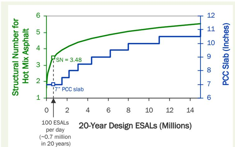
**Figure 1** Example pavement design process (shown for good soil)
