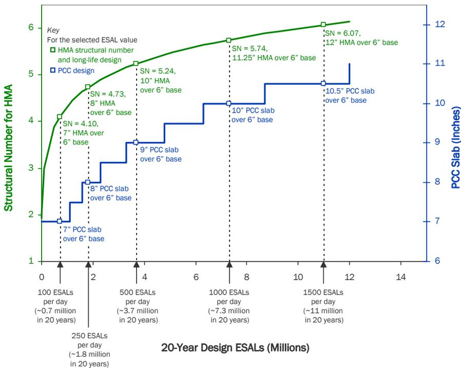
Figure 5 Pavement designs for poor soil
