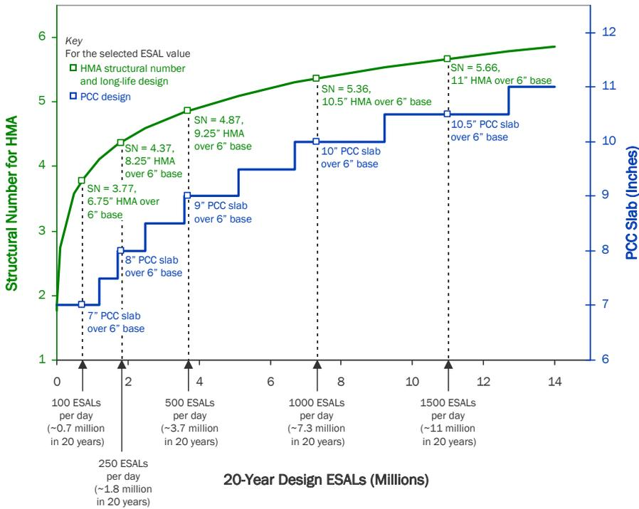
Figure 4 Pavement designs for moderate soil
