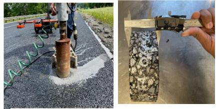
Find targets; measure thickness Core & confirm thickness
