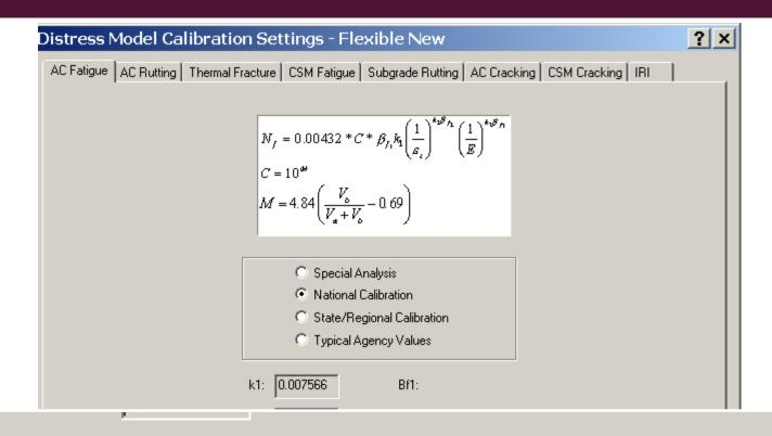
Endurance limit for calculation of HMA Fatigue Damage
