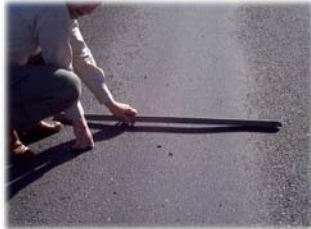
PG 67-22 unmodified, 15mm rut
