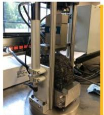
Image Source: FHWA Load Frame performing Ideal-RT
