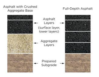
Figure 2.1. Asphalt Pavement Types
