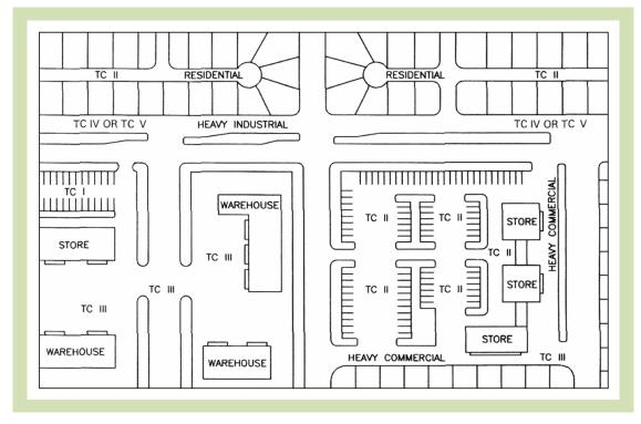
Figure 5.1. Typical Zones of Traffic Classes (TCs)
