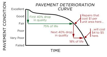
Figure 7.1. Relationship of Asphalt Deterioration and Rehabilitation
