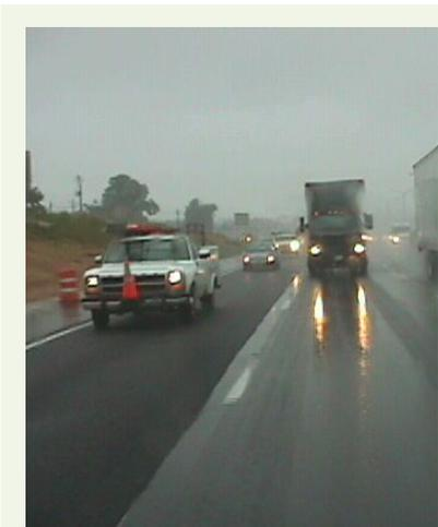
**Figure 6** The open graded friction course shown in the left lane reduces standing water and pavement noise. (Image courtesy of Asphalt Pavement Alliance)
