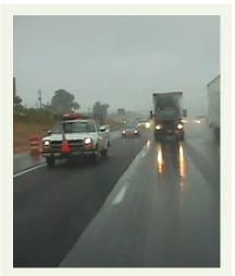
**Figure 6** The open graded friction course shown in the left lane reduces standing water and pavement noise. (Image courtesy of Asphalt Pavement Alliance)
