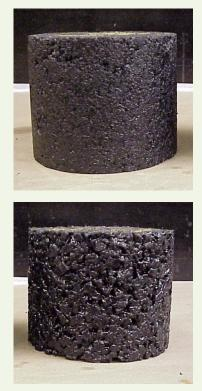
**Figure 4** Compared with densegraded asphalt (top), air voids in stone matrix asphalt (bottom) are more visibly apparent. (Image courtesy of the University of Washington)
