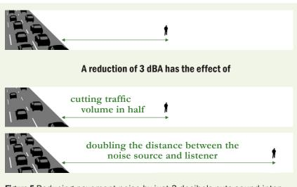
Figure 5 Reducing pavement noise by just 3 decibels cuts sound intensity in half.
