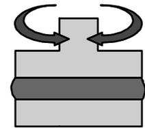
Test using the DSR applying a 1 sec creep stress followed by 9 sec recovery.
