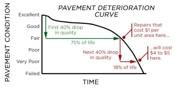
Figure 8.1. Relationship of Asphalt Deterioration and Rehabilitation
