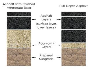
Figure 2.1. Asphalt Pavement Types
