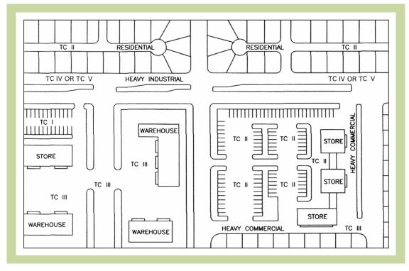
Figure 6.1. Typical Zones of Traffic Classes (TCs)
