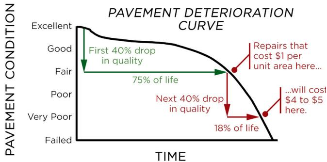
**Figure 8.1. Relationship of Asphalt Deterioration and Rehabilitation**
