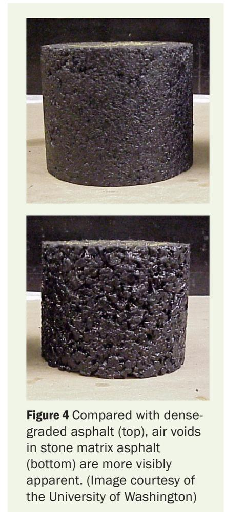
**Figure 4** Compared with dense-graded asphalt (top), air voids in stone matrix asphalt (bottom) are more visibly apparent. (Image courtesy of the University of Washington)
