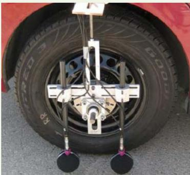
**Figure 2** Special equipment measures noise generated from the interaction of tires and the pavement. (Image courtesy of the Asphalt Institute)
