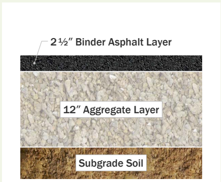
Figure 1 First-stage asphalt pavement used at the start of a subdivision project
