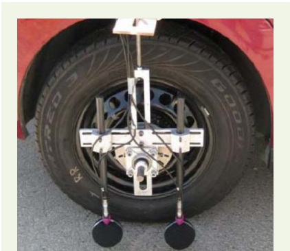
Figure 2 Special equipment measures noise generated from the interaction of tires and the pavement. (Image courtesy of the Asphalt Institute)
