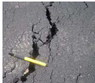
The hard way to learn about a weak subgrade or base. (Image courtesy of Transtec Group)
