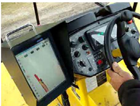
The pavement might be all black, but the readout of an IC system lets the operator know in living color the number of compaction passes. (Image courtesy of Sakai)
